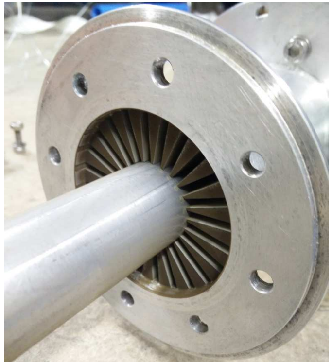
Fig. 12. Inner tube inserted into wire cut section
