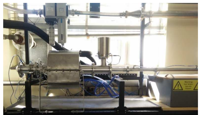
Fig. 4. Test section without insulation cladding
