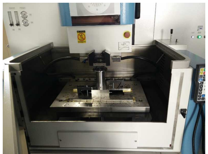
Fig. 10. Test section mounted in wire cutting machine
