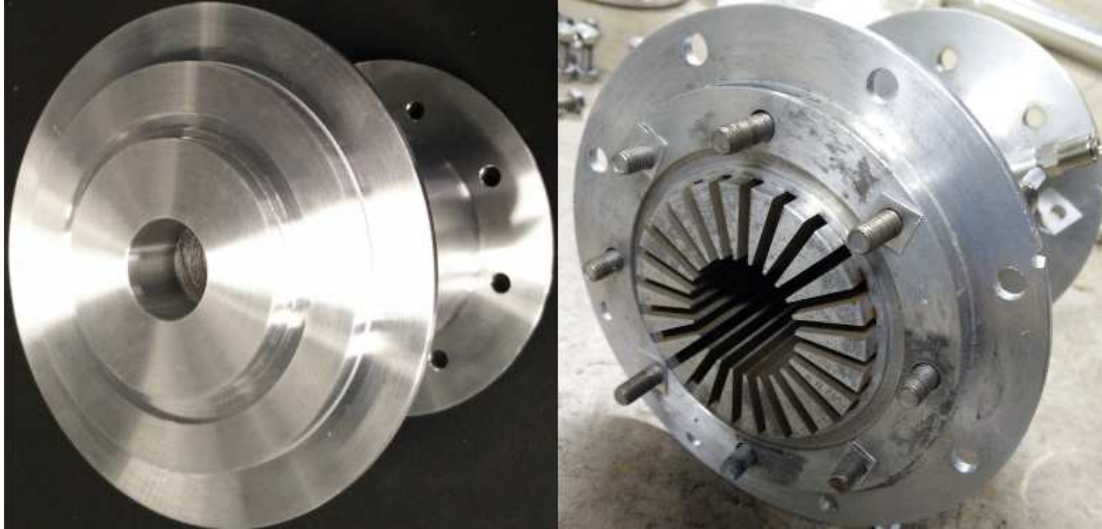
Fig. 11. Internally finned section before (left) and after wire cutting (right).
