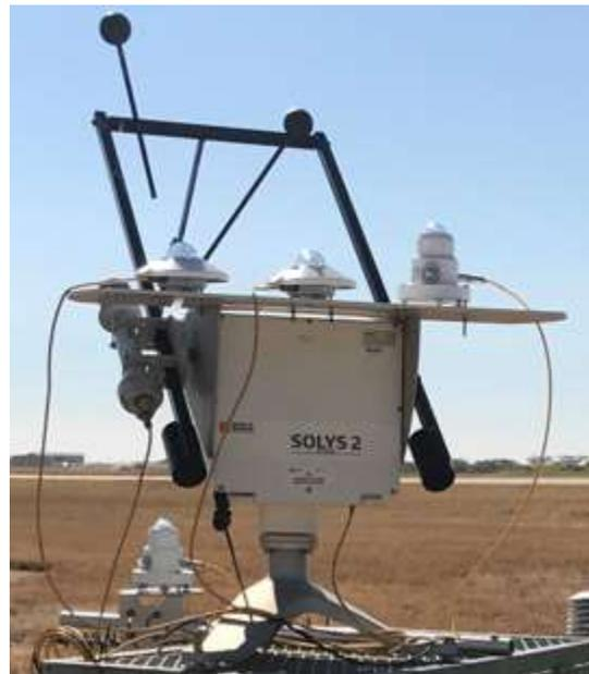
**Figure 1. Configuration of a SAWS radiometric station with an unshaded pyranometer at the centre.**
